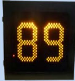
DF15 deployed in its stealth form (without front fascia) will blend into the background, only being seen when activated giving the biggest impact for the long term. Data can also be recorded in stealth mode to achieve a baseline of road speeds.
